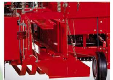
Rear wheel to help working on field with furrows
