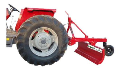
The Agro1's Adjustable Rear Blade with Grader Wheel, is the best tool to control the position of the Blade during Tractor operation. The Position and be controlled to hold the blade at the chosen depth for the fine leveling. Angle and Pitch of the Blade adjustable from. Tractor Seat. Blade Pitch is Adjustable from 0 — 40 Degree by the Screw Lever in reach of the tractor seat. The Blades can be completely reversed for back filling. For access to awkward place, it can be off set to either side.
