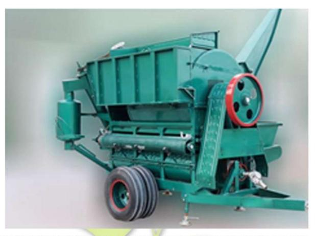
Rice / Paddy Thresher is tractor PTO driven and can be used with separate Diesel Engine as an option.
