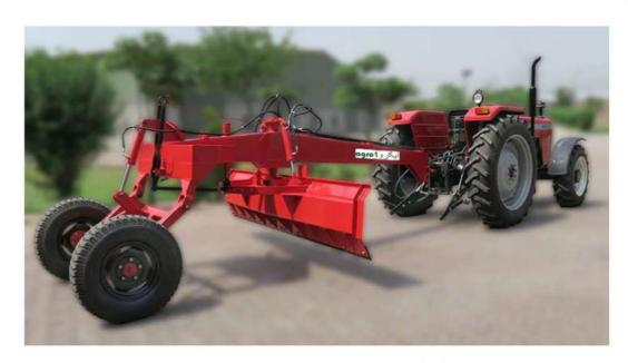
The Agriculture Leveling Drag or Rear Blade or Grader, that is developed with several adjustments that closely resemble a # motor grader. and designed to perform following works and applications.
