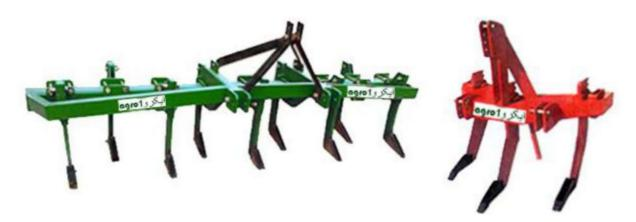
Its a primary tillage deep plough, working upto 20 inches to ensure development of crop root system at proper depth and environment. It is ideal to implement where topsoil is fertile but subsoil is not productive.
